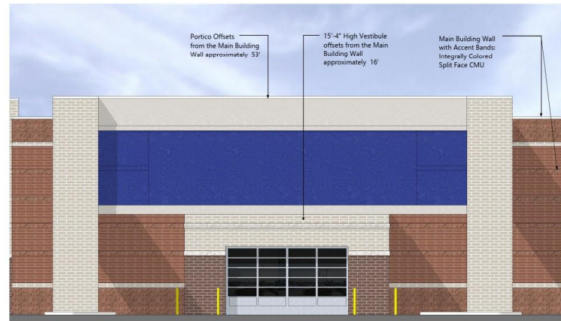
WEST ELEVATION - PROSERVICES ENTRANCE
