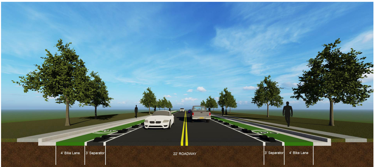
FIGURE 6.6: CONVERTED NEIGHBORHOOD STREET SECTION WITH BIKE LANES
