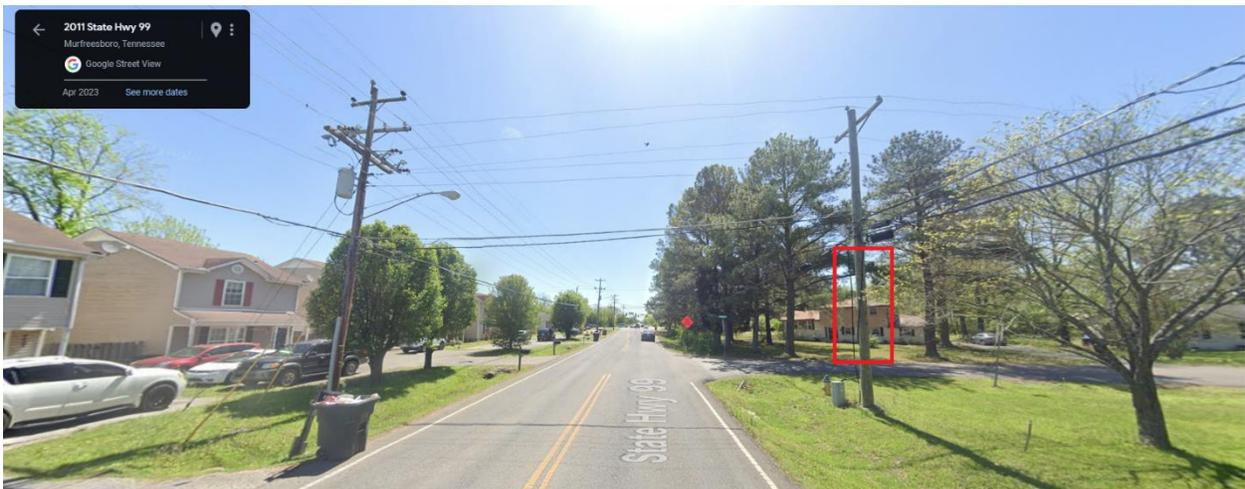
Camera 23 EB SR 99 @ S Rutherford Blvd to be installed on existing power pole.
